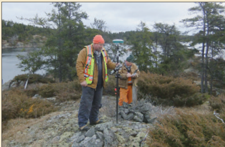
Bob Halliday (left) taking an RTK measurement with crew member Murray Dawson
